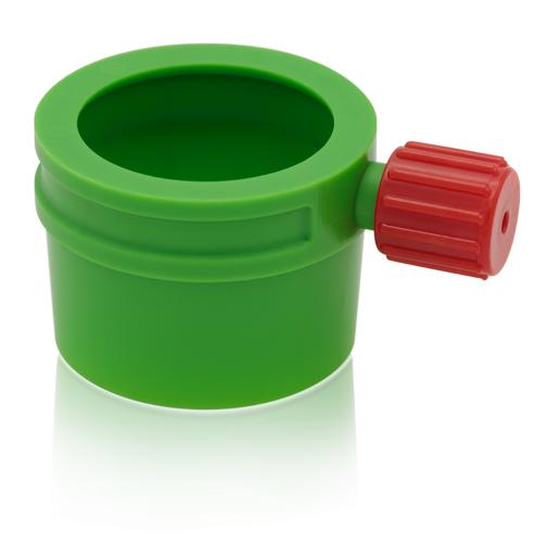
The Connector Ring is a sterile device to support active filtration, cell detachment, cell lysis or cell stimulation in combination with a pluriStrainer and a 50ml standard (conical) centrifuge tube. pluriStrainer, Connector Ring and a 50ml tube can be combined to a unit. This unit allows for a controlled flow through the sieve. When the Luer-lock of the Connector Ring is closed, sample or liquid remains on the sieve. An open Luer-lock starts the separation or the filtration process.
