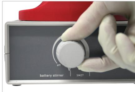
After completing the mixing procedure, switch off the magnetic stirrer, remove the sample holder from pluriPlix® and remove the reaction tubes from the sample holder.
