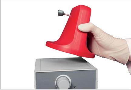
Place the pluriPlix® mixer on a magnetic stirrer. Make sure that the heating unit of your magnetic stirrer is turned off and cooled off. Position the mixer in the center of the magnetic stirrer so that the magnetic force of the stirrer is optimally transferred to the pluriPlix® drive shaft.
