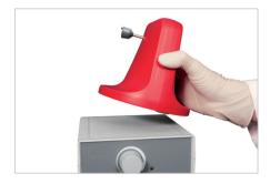
Place the pluriPlix<sup>®</sup> mixer on a magnetic stirrer. Make sure that the heating unit of your magnetic stirrer is turned off and cooled off. Position the mixer in the center of the magnetic stirrer so that the magnetic force of the stirrer is optimally transferred to the pluri-Plix<sup>®</sup> drive shaft.
