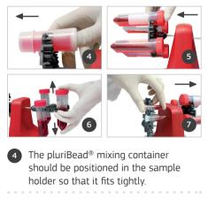
Lids of larger reaction tubes (e.g. 50 ml tubes) should face the pluriPlix<sup>®</sup> housing. Adjust the lids close to the sample holder to avoid blocking of the rotation.
